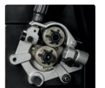
Heavy-duty aluminum two-drive-roll system
