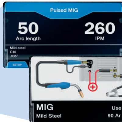
Pulsed MIG setup screen
