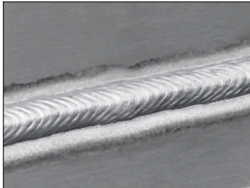
Pulse-On-Pulse on 3 mm Aluminum
